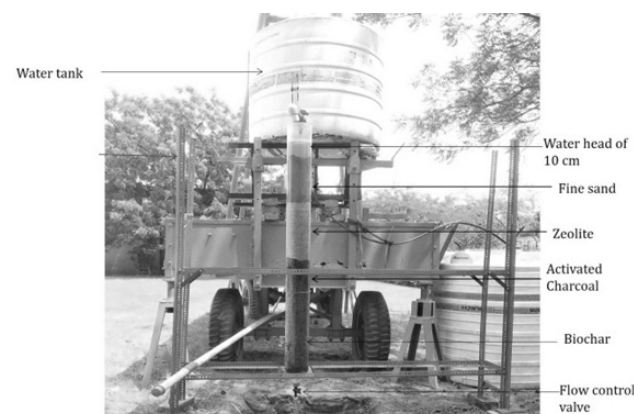
Fig. 1. Installation of combination of filter media
