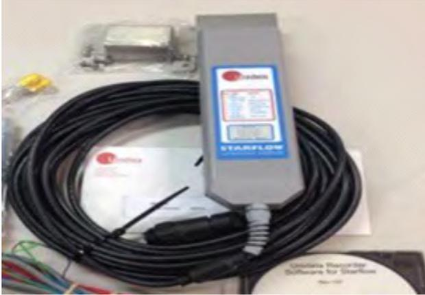
Fig. 3. Ultrasonic Starflow meter for inflow measurement
