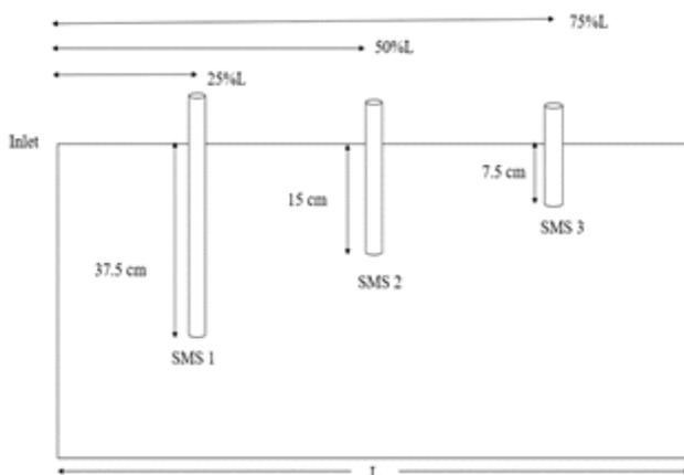
Fig. 1. Placement of soil moisture sensor in the field
