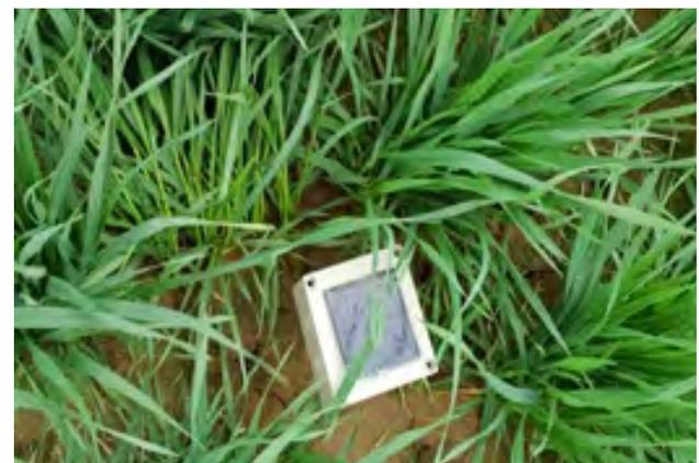
Fig. 2. Soil moisture sensor under wheat crop in basin layout during *rabi* cropping season 2019-20
