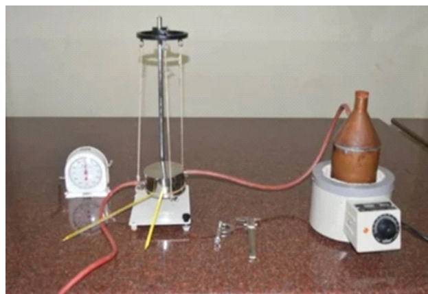
FIGURE 2 Thermal conductivity - Lee's Disc apparatus experimental setup
