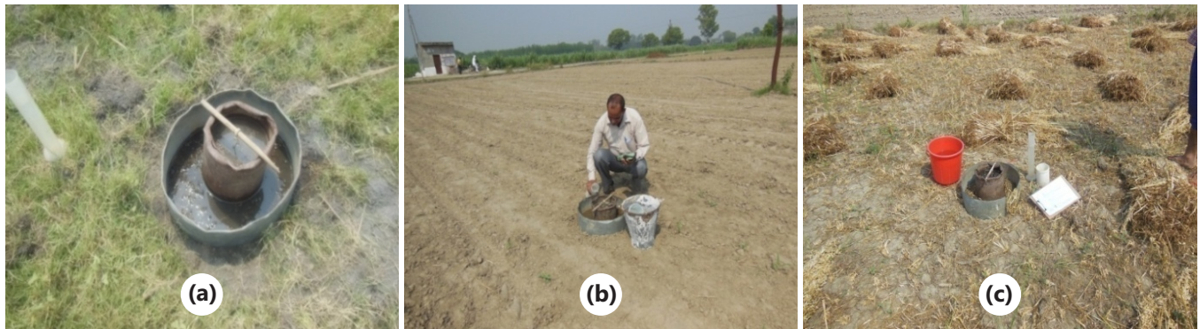
Fig. 8. Infiltration study at different locations, (a) in Harsauli drain, (b and c) in cultivated land
