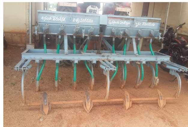
Fig. 1. Tractor drawn Ananta planter with attached shovels for formation of CF at the time of sowing (CF at 45 cm apart at the time of sowing)
