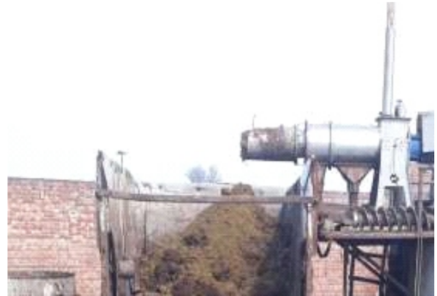
(b) Digestate coming out of the digester
