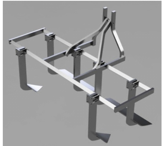
Fig. 4. Isometric view of the low hp tractor drawn intercultivator cum conservation furrow opener
