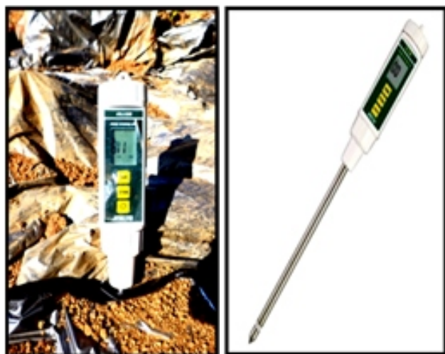
Measurement range: 0% to 50% moisture content of soil sample with 0.1% resolution
