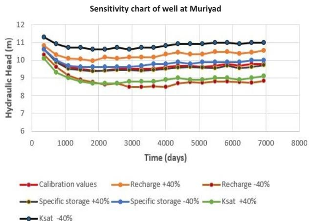
Fig. 9. Sensitivity chart of observation well at Muriyad
