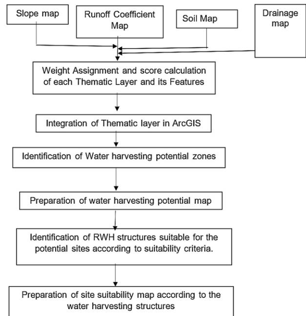
Fig. 3. Flow chart to identify the Suitable sites for RWH structures
